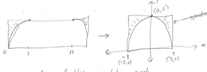
Equation of the parabolic arch
